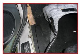
Lift front section of carpet and run wire beneath carpet and up to centre console.
