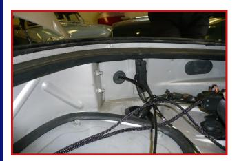
Route long part of harness through grommet on left hand side just above car main harness grommet. You will need to make a hole in original grommet.
