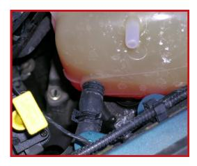
Clip the sensor to the bottom of the new expansion tank and fit the two supplied metal tubes into the plastic tank pipes as this will help to prevent the pipes from crushing when tightening the hose clips. Then refit tank in reverse order. Then top up with fluid from the old tank. You may find in necessary to top up with new anti-freeze/water mixture.
