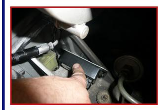
Secure ECU to triangular reinforcement section on left hand side of boot, with the aid of fir tree clip and double sided tape.
